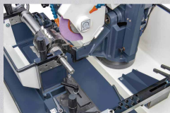
G320PS Multiple tracing rods allow for accurate and convenient grinding
