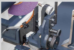
G320PS Grinding wheel dressing
