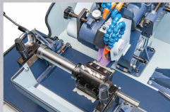
G320P Profile knife grinding
