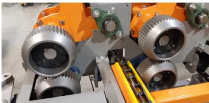
MFE-300 FEEDING WHEELS MADE OF STEEL WITH HARDENED SURFACES TEETH
