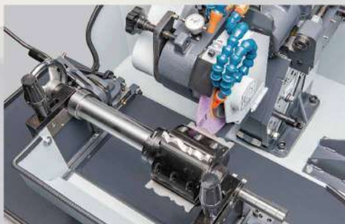
G320P Profile knife grinding
