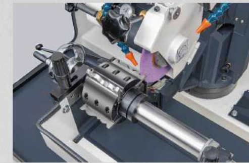
G320PS Profile knife grinding
