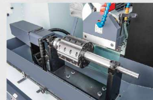
G320A Knife Edge Grinding (Movable straight knife)
